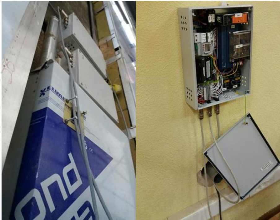
Figure 3: (left) 2 devices installed inside the ventilated façade and (right) one device indoors, showing the internal elements.
